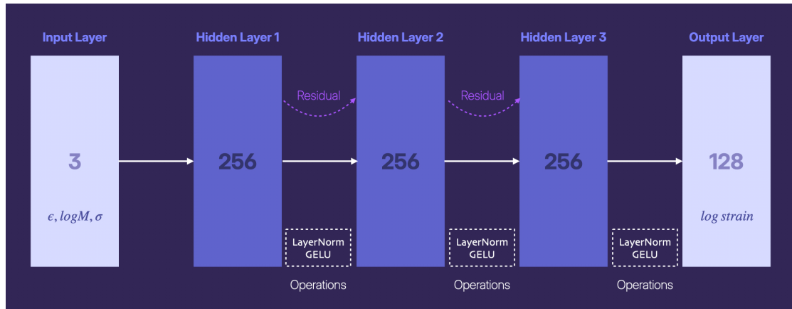
FIGURE 4.1: Architecture of the NN emulator with three input parameters, three uniform hidden layers (256 neurons each) with residual connections, and a 128-dimensional log-strain output. LayerNorm and GELU activations are applied after each hidden layer.
